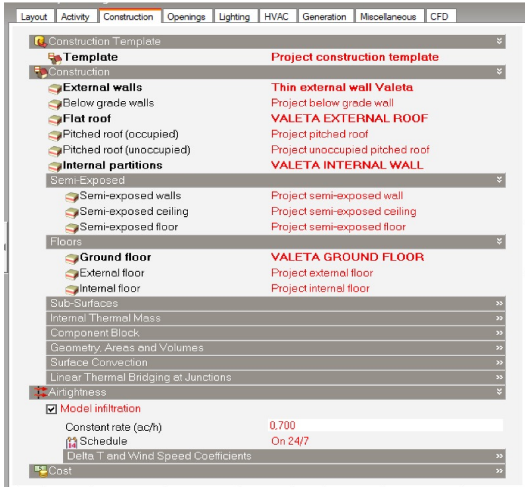
Figure 18. Construction Templates definition and Airtightness
