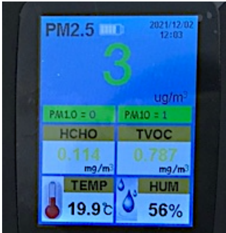
Figure 61. Particle counter in an office with high levels of TVOC and HCHO
