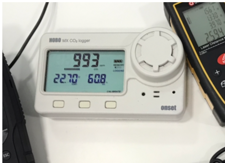
Figure 59. High concentration of CO 2 in an office
