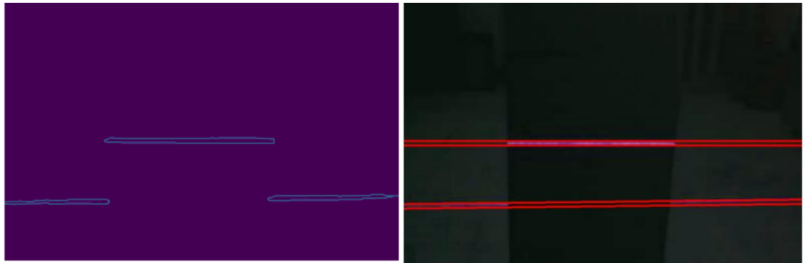
Fig. 25. Canny image and result image with lines detected.
