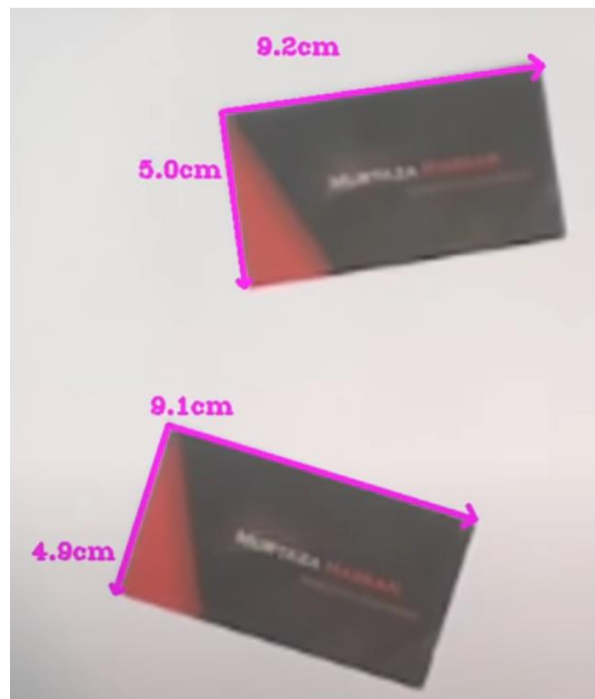
Fig. 2.7. Measuring distances with a camera vision system.
