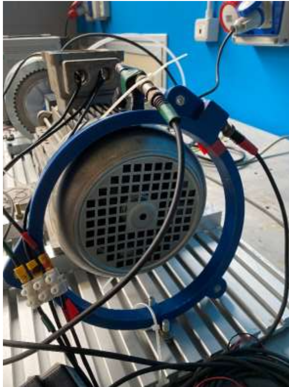
Figure 42: Emerson M 343 F - 1204, on the rear of the RAEL induction motor
