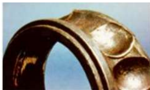
Figure 18: Plastic deformation on an inner ring raceway produced by overloading (RKB, 2010)
