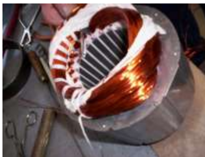
Figure 1: Stator windings (Frosini, 2022)
