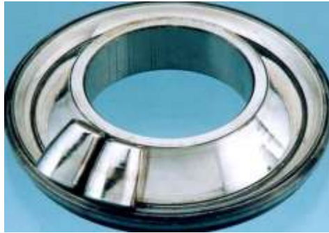
Figure 17: Bearing failure due to improper mounting (RKB, 2010)
