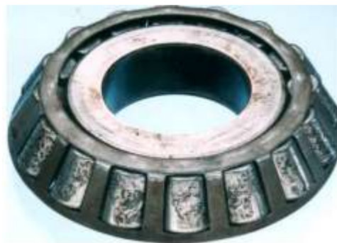
Figure 20: Bearing failure due to water contamination (RKB, 2010)
