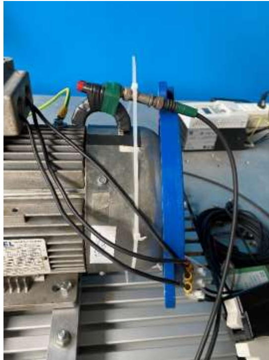
Figure 43: custom flux-probe for radial flux
