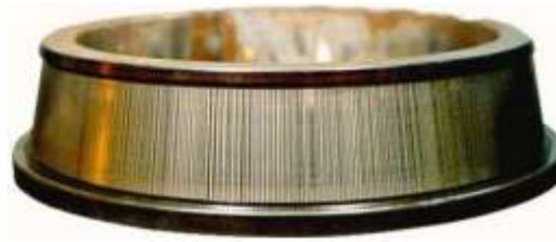
Figure 19: Craters formed by current leakage resulting in fluting (RKB, 2010)
