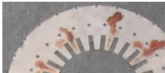
Figure 13: interlaminar insulation failure (Lee, 2021)
