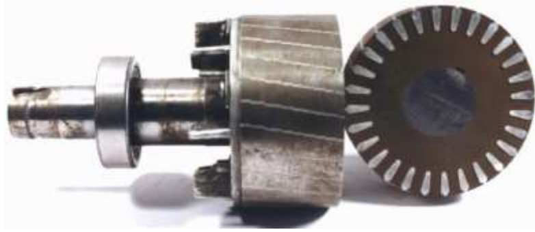
Figure 3: Squirrel Cage rotor (Frosini, 2022)
