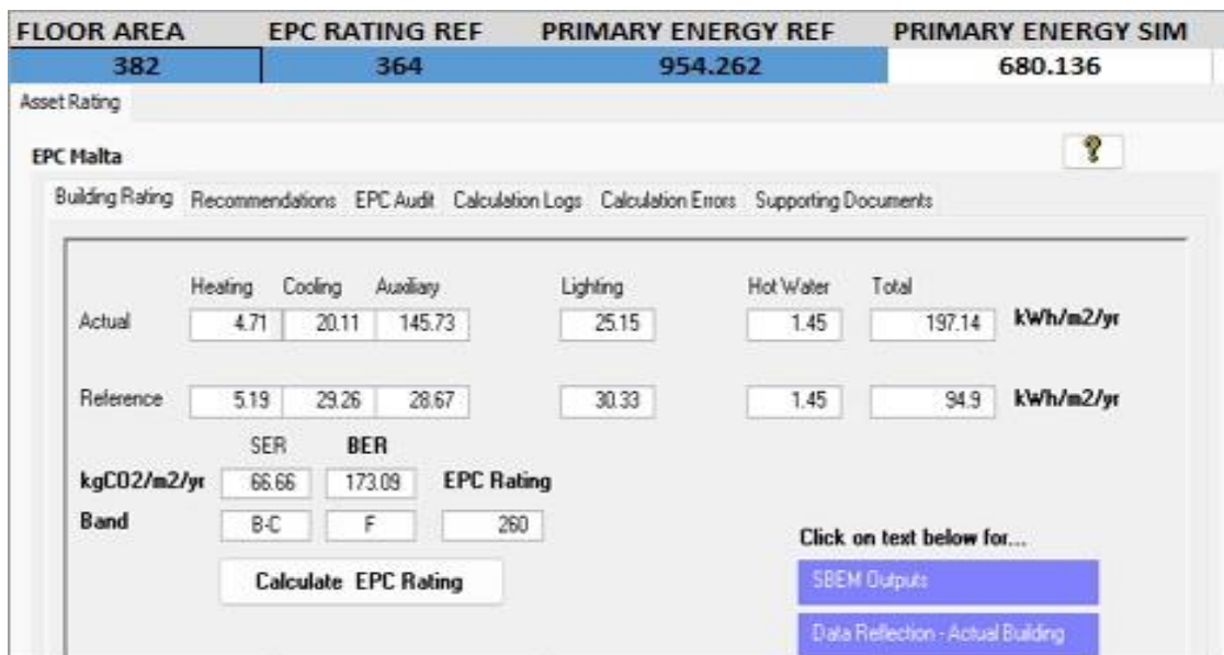
Figure 87. EPC Rating results for all measures less PV systems in 104 m2 Reference Building, SBEM-mt.
