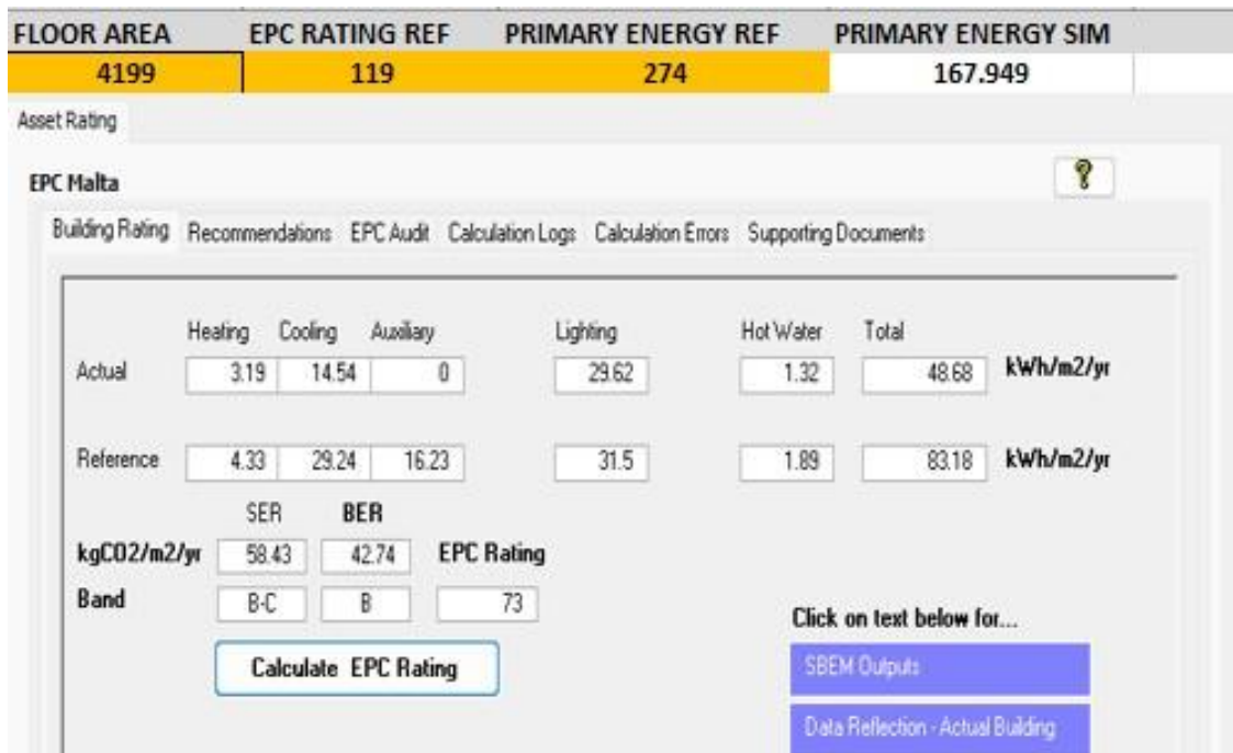
Figure 111. EPC Rating results for all measures less PV systems in 4199 m2 Reference Building, SBEM-mt.
