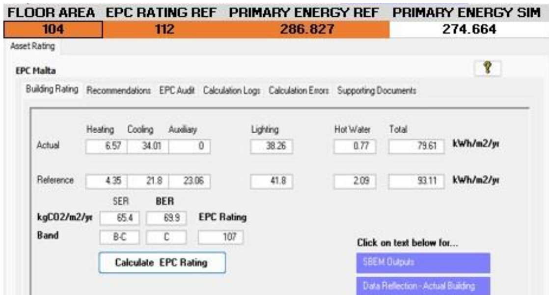
Figure 72. EPC Rating results for walls, roof and glazing for 104 m2 Reference Building after applying the best percentage improvements measures, SBEM-mt.
