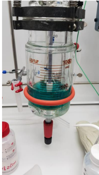
Figure 21. Reactor with homogeneous catalyst
