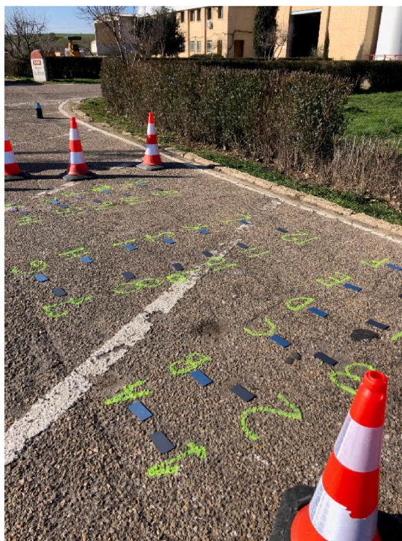
Fig. 4. Open-field experiments with carbon and galvanized steel probes.
