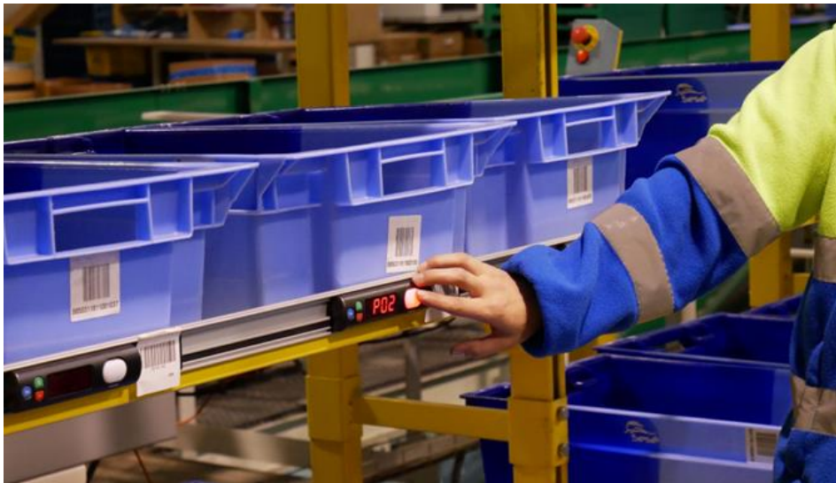
Figura 20: Operario utilizando dispositivo de Picking (Pick to light systems, 2022)
