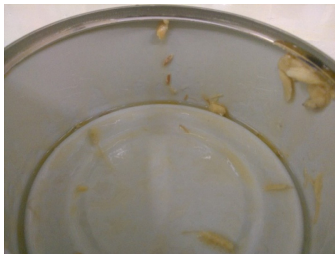
Figure 1. Muscle residues adhered to PET polymer after emptying the container. Areas of polymer coating with and without salmon adhesion.
