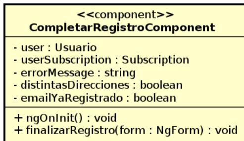
Figura 7.48: CompletarRegistroComponent class
