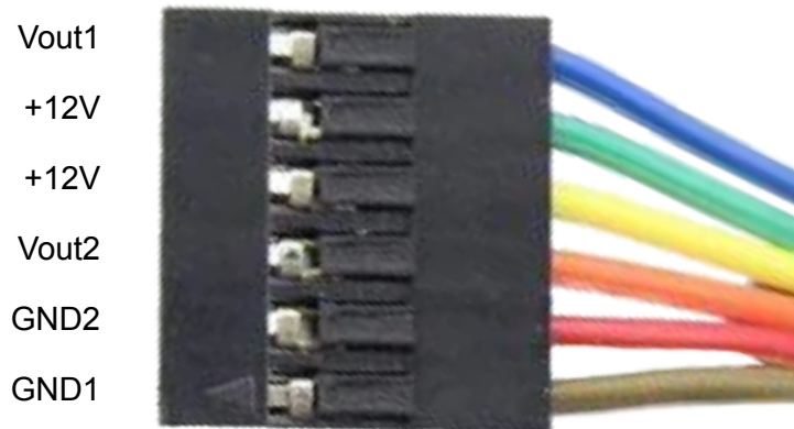
Figure 23. Wires going to the pedal.
