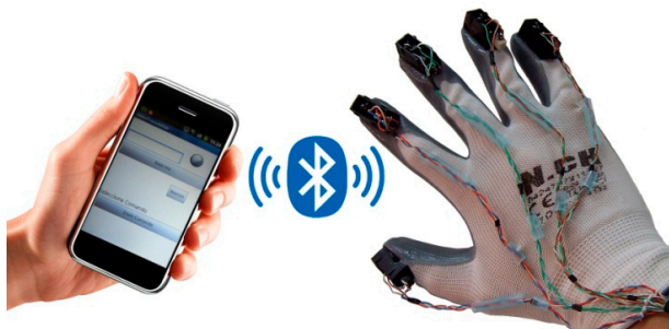
Figure 1. Communication system: (i) smartphone as afferent human-machine interface (HMI) for the unimpaired interlocutor, (ii) stimulating glove as efferent HMI for the deaf-blind individual, and (iii) Bluetooth link.
