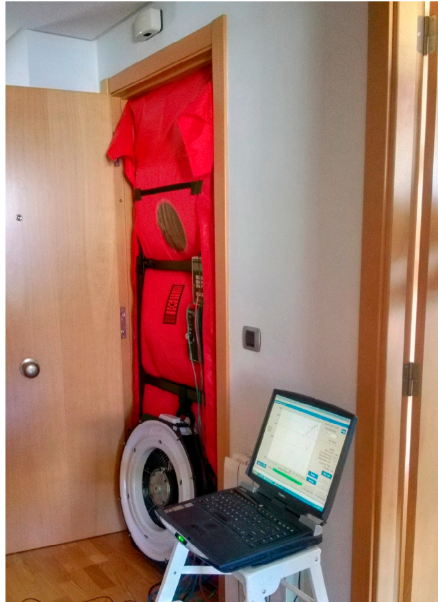
Figure 2. Blower door system.
