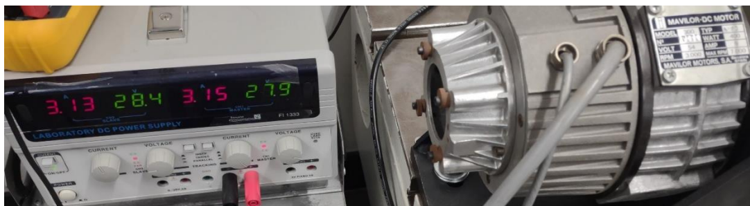
Figure 14: Limite de l'alimentation de laboratoire (protection constant current)
