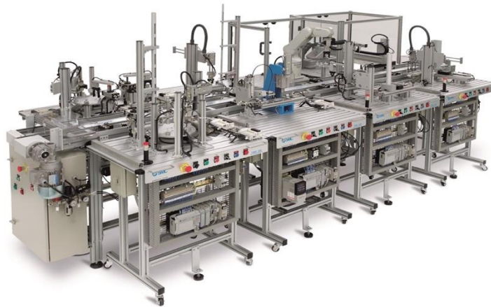
Figure 1. FMS-200 lineal transfer layout with 8 modules
