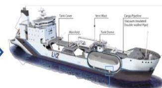
KHI LH<sub>2</sub> transport 88.5 tonnes LH<sub>2</sub> from Victoria to Japan in 16 days
