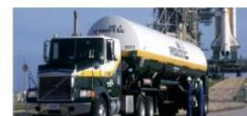
Air Products LH<sub>2</sub> tanker, 0.4-6.7 tonnes LH<sub>2</sub>
