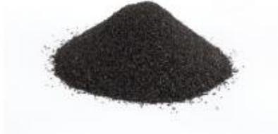
12kg H<sub>2</sub> at 20K with 37.5kg catalyst, takes 4.75mins to reach 99.8% para-hydrogen
