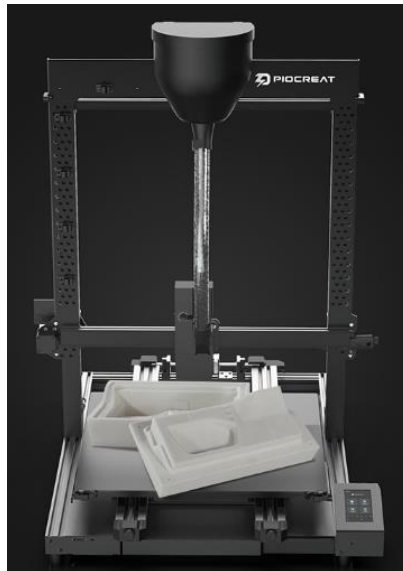
Figura 27: Impresora 3D Piocrete G5 Industrial FGF Pellets 3D Printer.[9]
