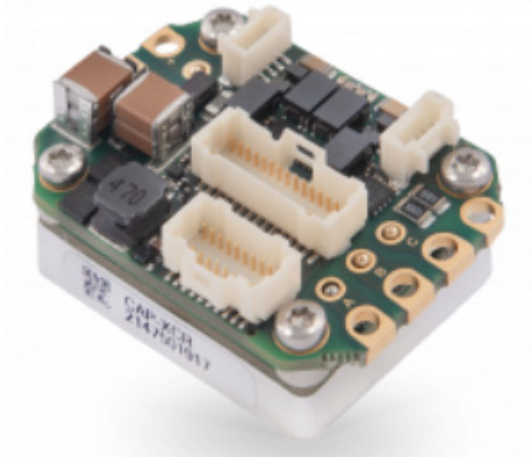
Fig. 62. Capitan XCR CANOpen de Novanta Drives. [38]
