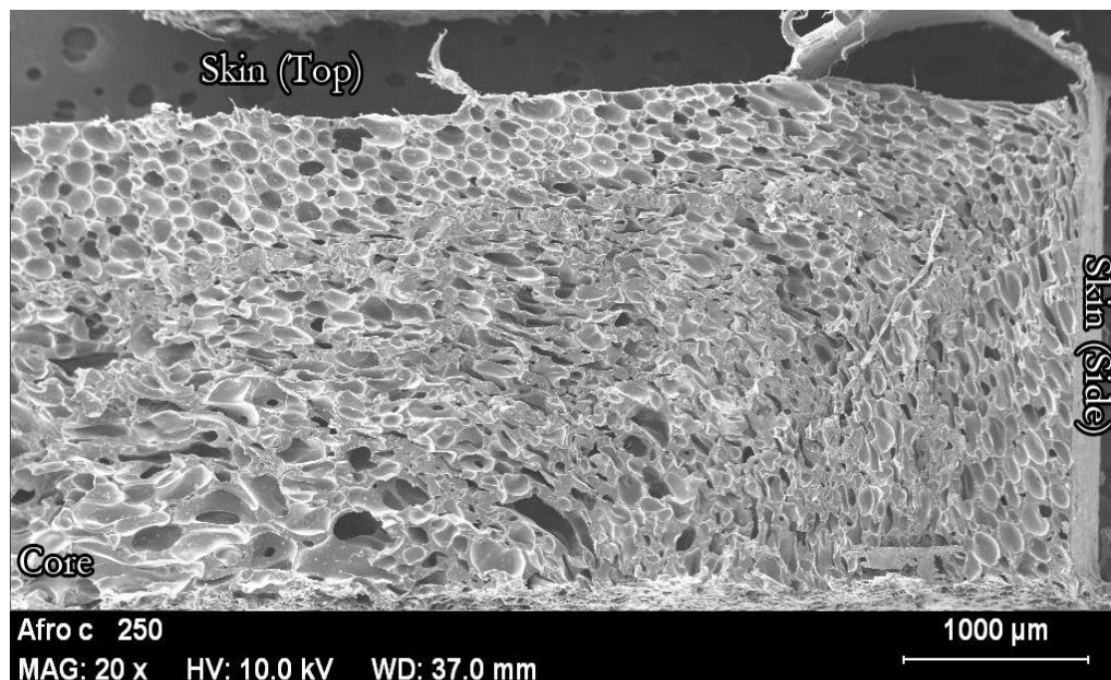
Figure 13. Sample with a relative density of 0.2 and produced with 10.5% of azodicarbonamide. Near the skin the cellular structure shows a regular structure. 500μm from the skin, several cells are crushed in the direction from the core to the skin. In the core, the cells are four times larger than in the skin.
