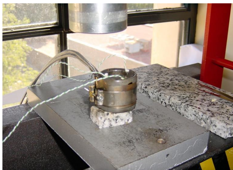
Figure 3. Experimental setup of mold with all the thermocouples in the mold to control the temperature.
