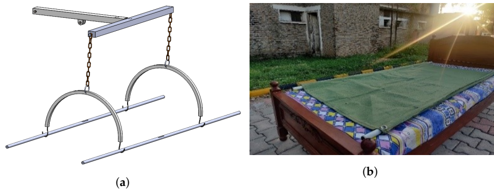
Figure 7. (a) Upper frame and (b) stretcher assembly.
