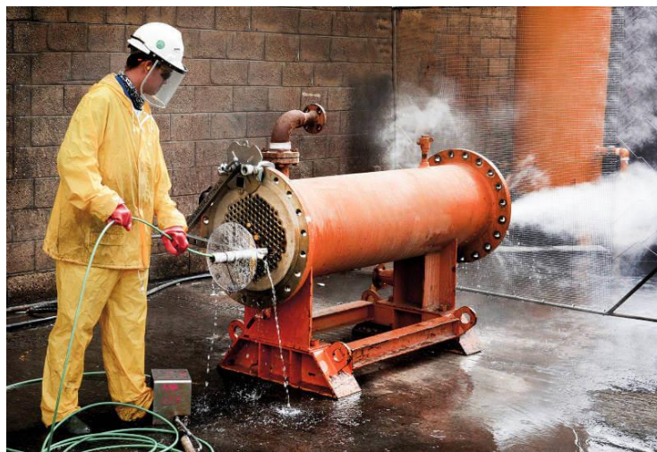
Figure 4. Conditioning process of a heat exchanger
