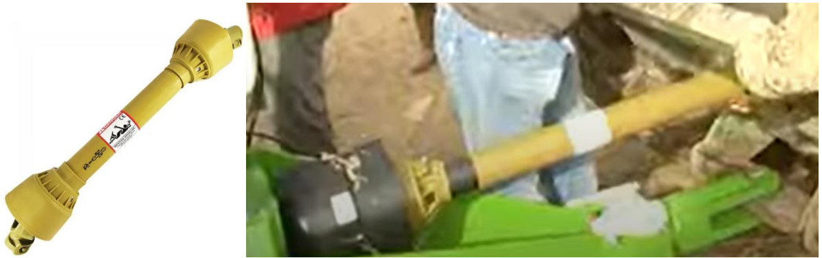
Fig. 1.15: Cardan join and power take off ( https://www.tractoresymaquinas.com/transmision-de-potencia-en-el-tractor/ )
