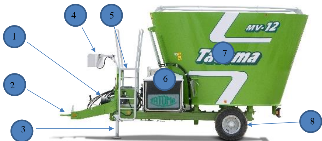
Fig. 1.13: Vertical Mixer with one endless screw and conveyor belt MV-8 10 12 14 16 18; 1 – Power take-off; 2 – Hook; 3 – Hydraulic base; 4 – Manual controller; 5 – Leader; 6 –
