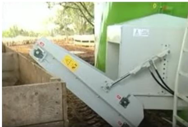
Fig. 1.20: Additional conveyor belt with adjustable height ( https://www.youtube.com/watch?v=WRDfR5v2OO8&list=UU2T_U1o_MWTGGTD2r-M9MhQ )
