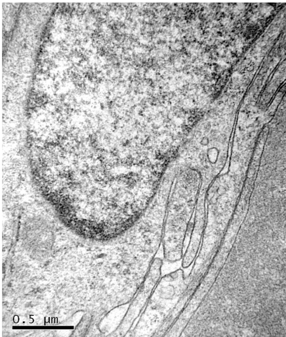
Image 7.1. Transmission microscopy evidencing the Epithelial cell Membrane being attached to the SF-PEG membrane surface
