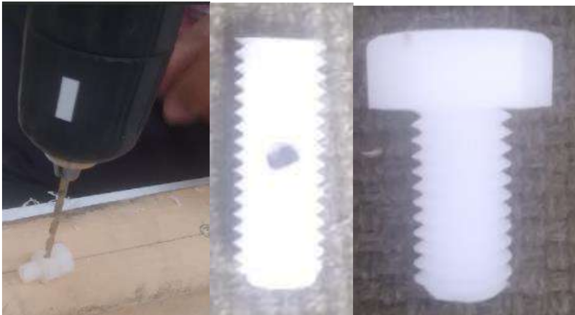
Figure 25 : Drilling nylon screw process
