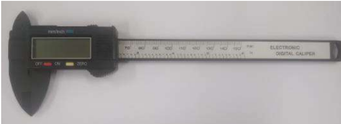
Electronic digital calliper with an accuracy of +/- 0,1 mm
