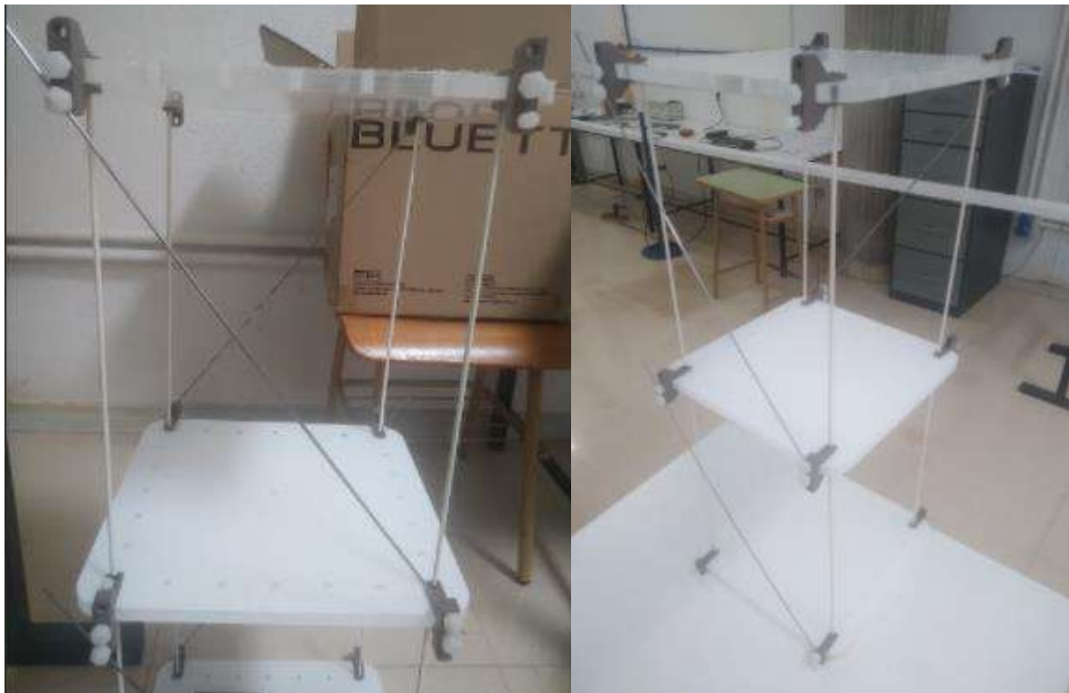
Figure 49 : Diagonal configuration of the 3D building
