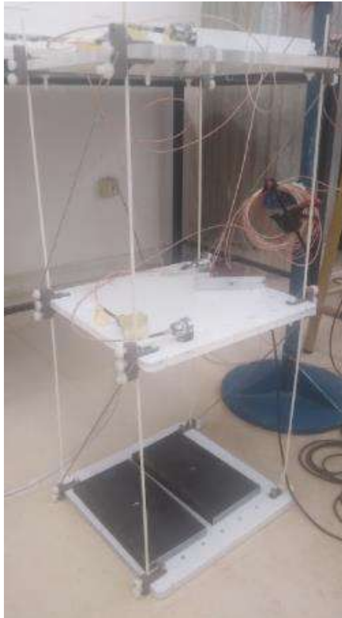
Figure 69 : Diagonal bracing configuration building
