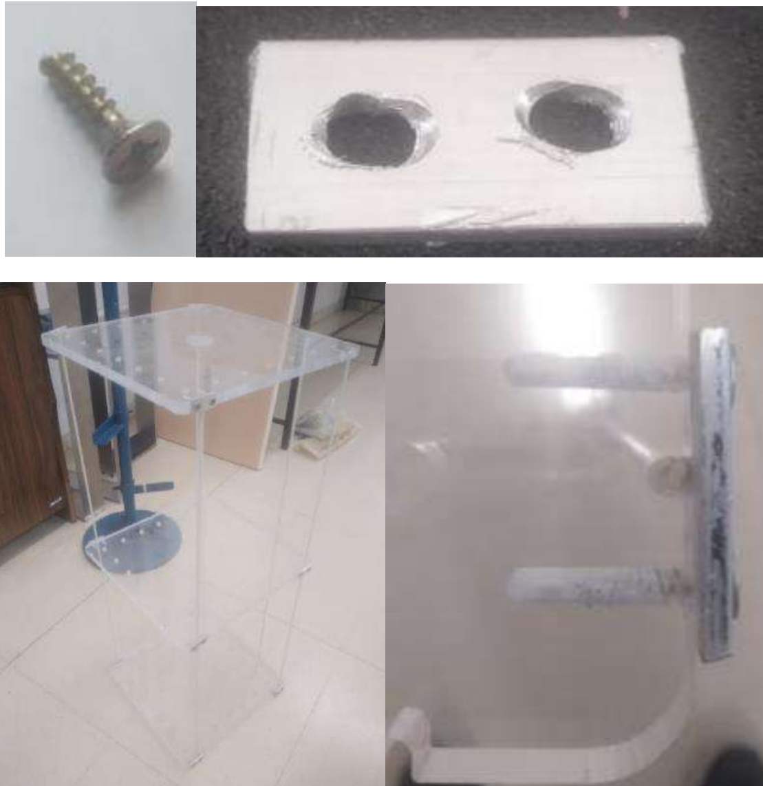
Figure 5 : Old solution with aluminium plate and cut screws
