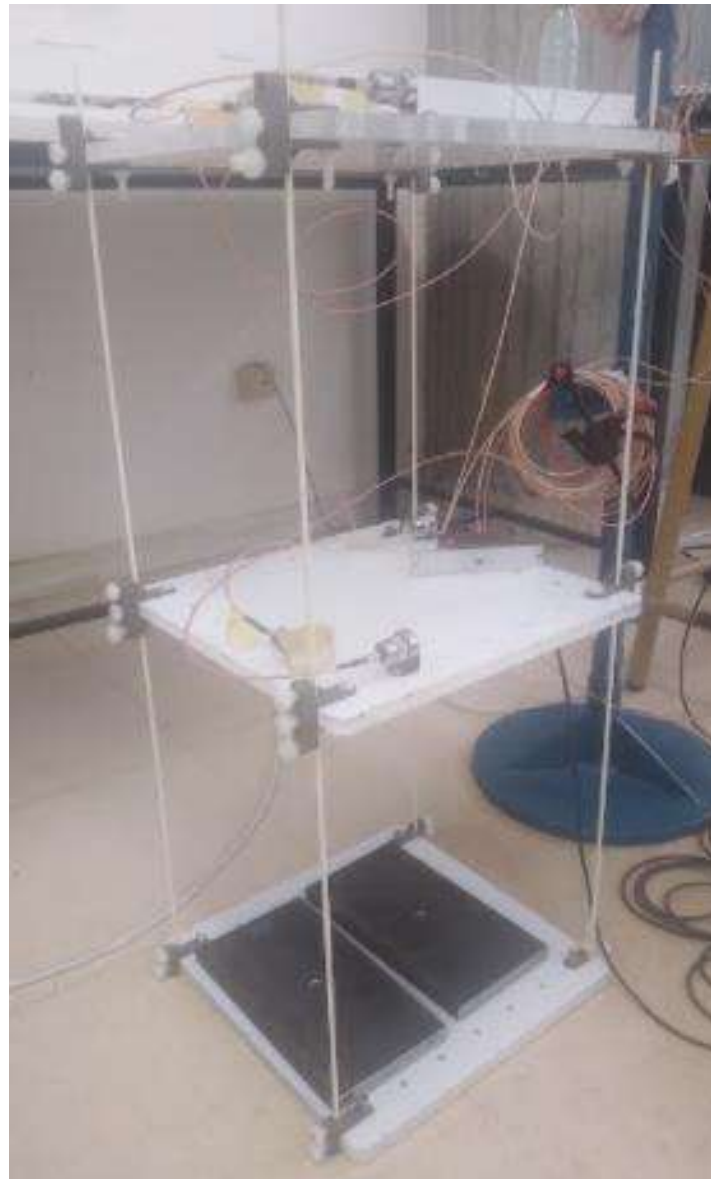
Figure 67 : Without bracing configuration building
