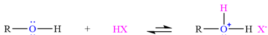
Figure 5.1: Protonation of an alcohol by an acid which produces an oxonium ion.
