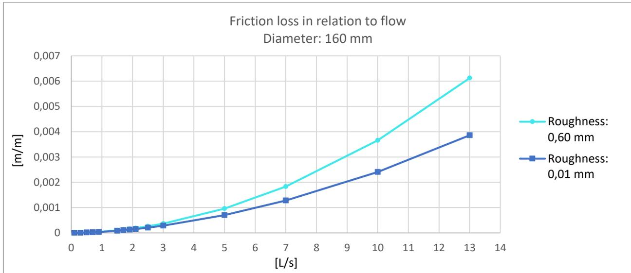
Figure 8.10 Friction loss in relation to flow at different roughness, diameter of 160 mm.
