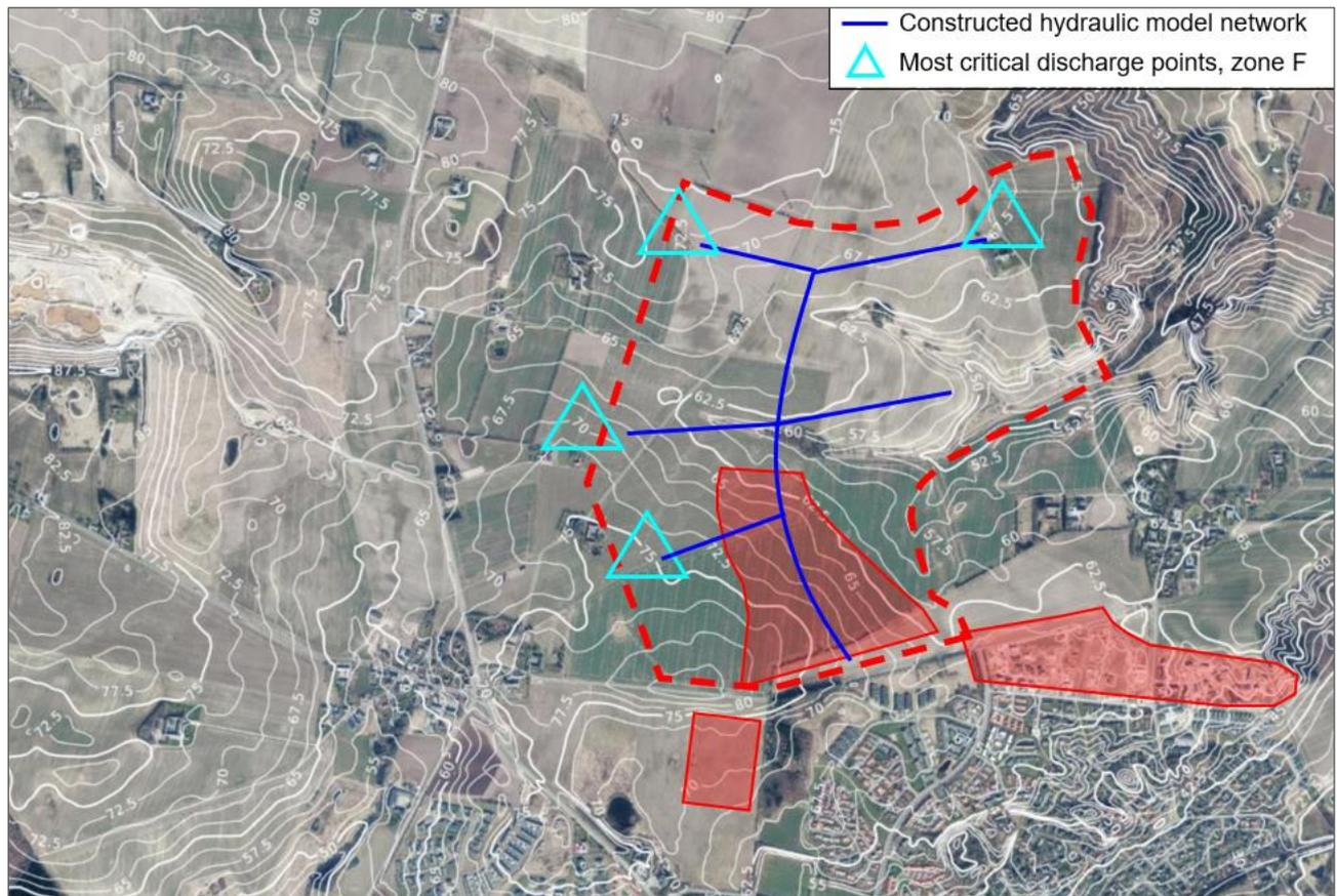
Figure 9.4 Overview of constructed hydraulic model network and identified most critical future discharge points, Scalgo LIVE.
