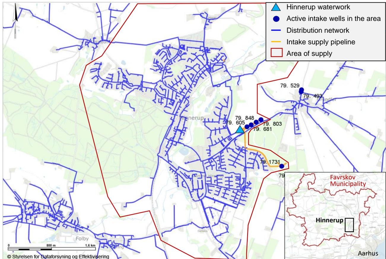
Figure 5.2 Overview of supply network, waterwork and active intake wells, (Favrskov Vandforsyningsplan (2020-30), 2020).
