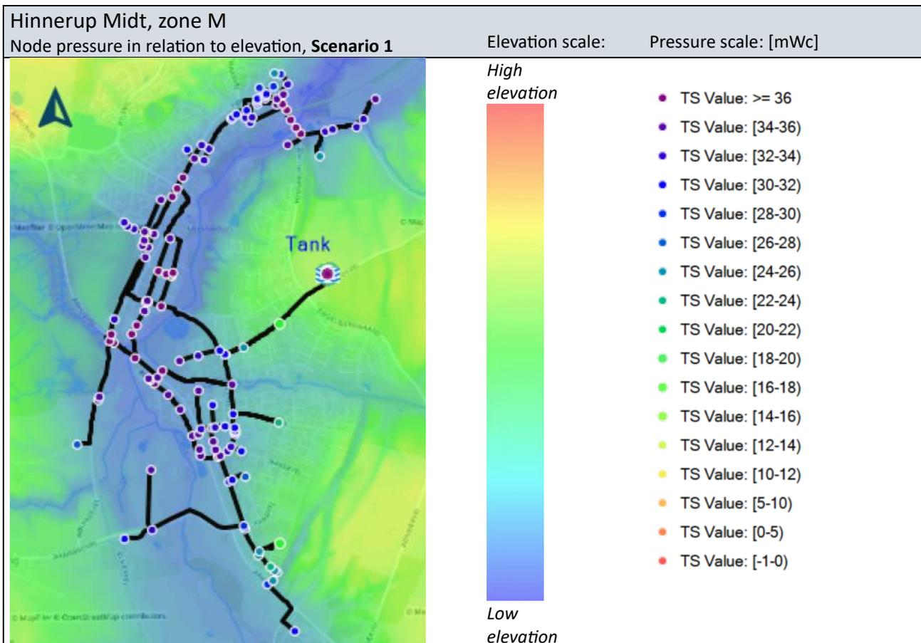
Figure 8.13 Hinnerup Midt, zone M, node pressure in relation to elevation, Scenario 1
