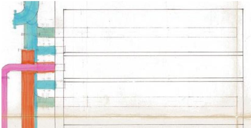
Figure 7.8 The top view of one of the eight sand filters in Hinnerup showcases color-coded pipes entering and exiting the filter. The raw water flow is indicated by the color red, the clean water flow is marked in blue, the backwash water is represented by green, and the pink pipe is used for air ventilation during the backwashing process. Excerpt from drawing provided by the waterworks.
