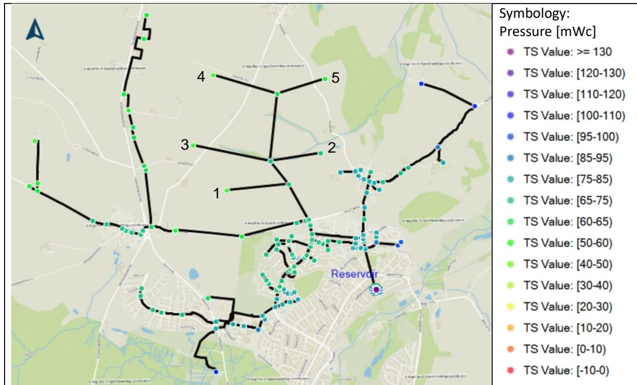
Figure 9.5 Consumer pressure at critical discharge points for future zone F and current zone R when zone F is connected. Result of hydraulic modeling.
