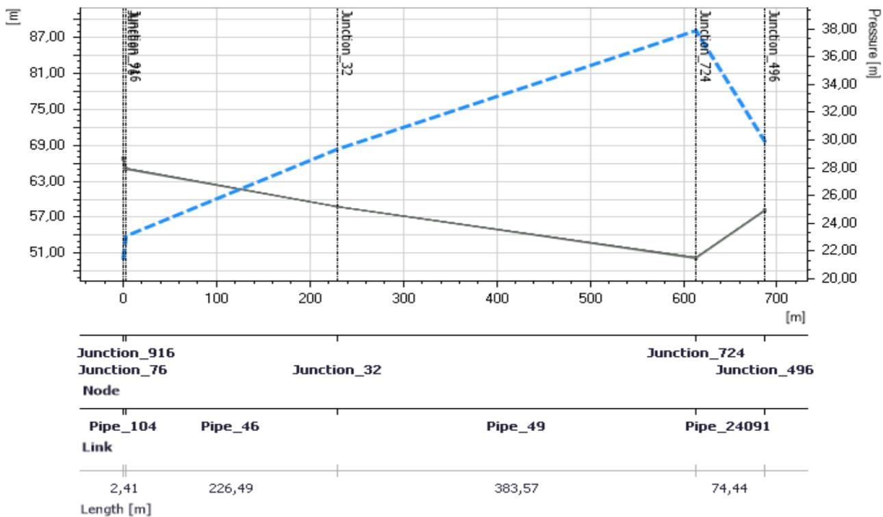
Figure 8.17 Profile plot of change in pressure. Water moving from main supply pipe to identified critical discharge point within the zone.
