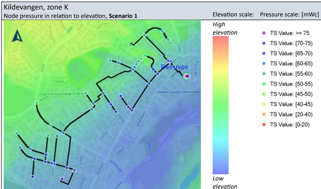
Figure 8.14 Kildevangen, zone K, node pressure in relation to elevation, Scenario 1
