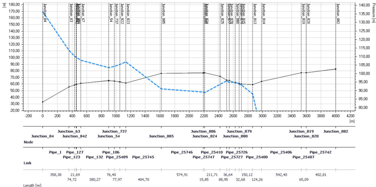
Figure 8.22 Profile plot of change in pressure. Water moving from main supply pipe to identified critical discharge point within the zone
