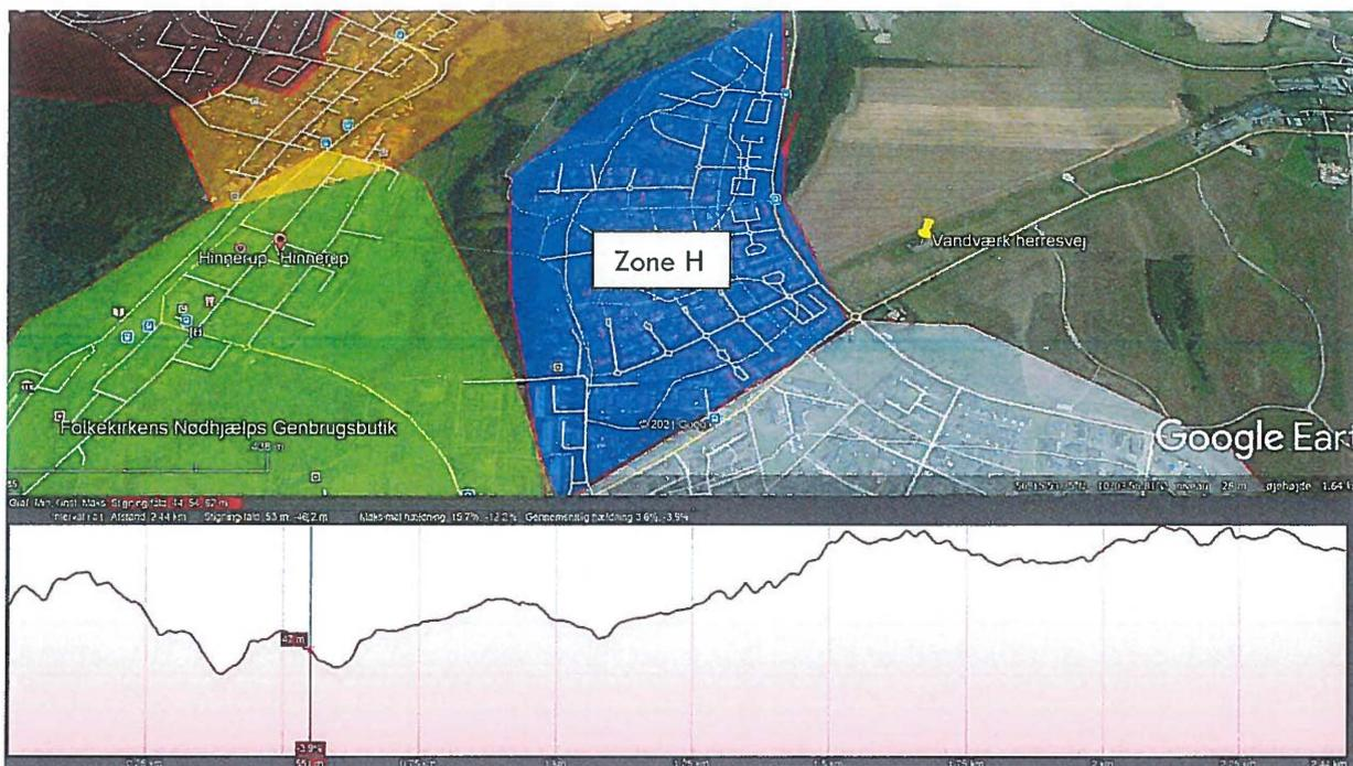
Hinnerup Lund zone H. There is an elevation difference from level 62 to level 44, equal to a difference of 18 meter.
