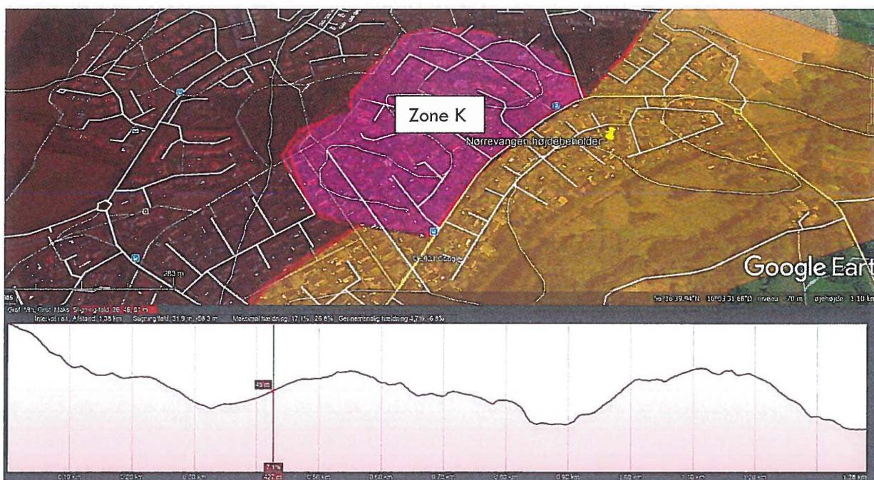
Kildevangen zone K span from level 60 to level 36, equal to a difference in altitude of 24 meter.
