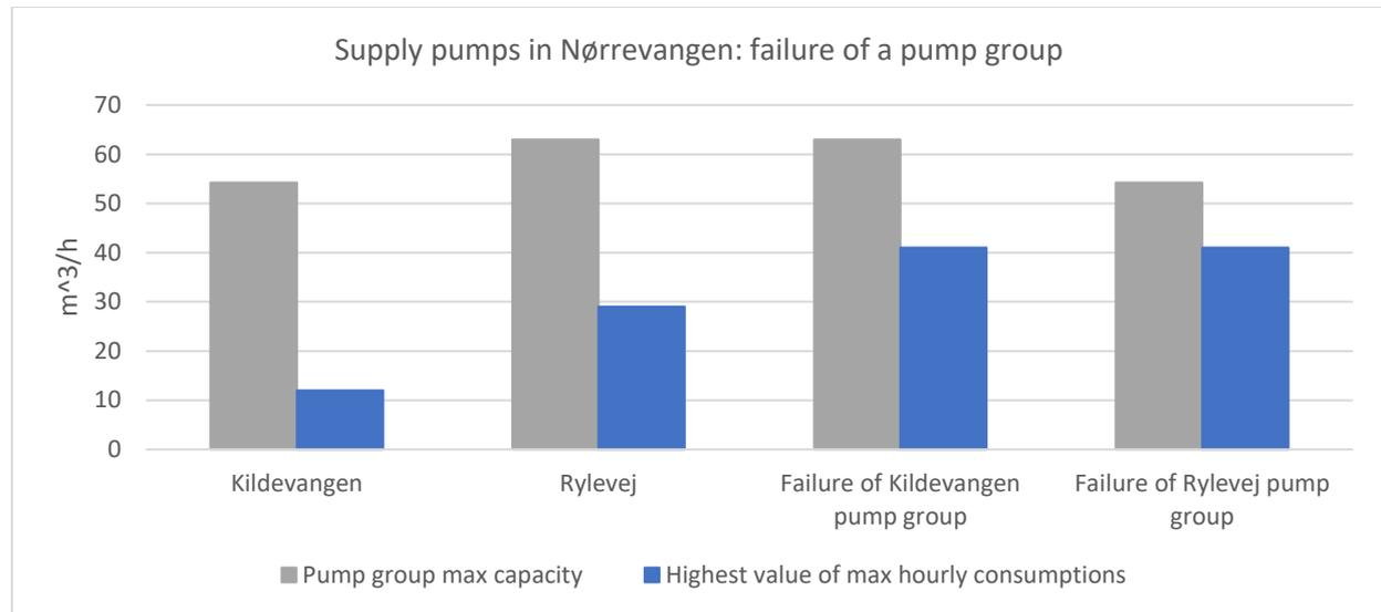
Figure 10.2. Pump capacity vs. Maximum hourly flow to provide in different scenarios.
