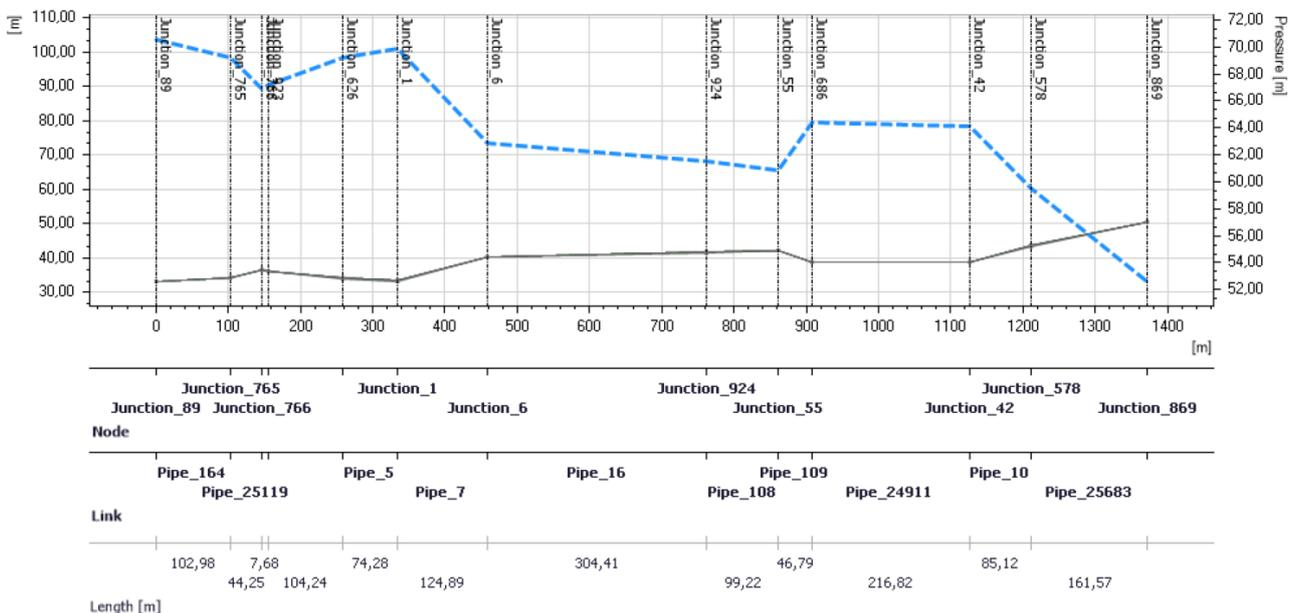
Figure 8.20 Profile plot of change in pressure. Water moving from main supply pipe to identified critical discharge point within the zone
