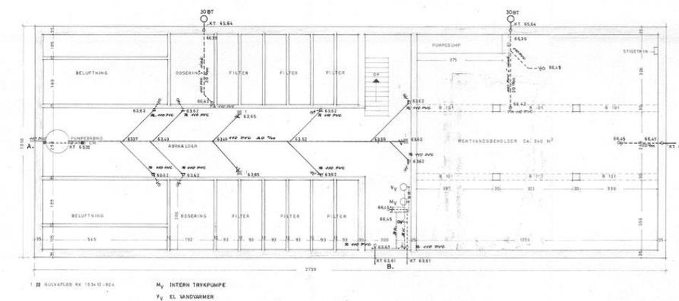
Figure 7.11 Schematic drawing of the floor plan in the Hinnerup waterworks. The drawing is not quite up to date, the "Dosing" has now also been converted into a sand filter.
