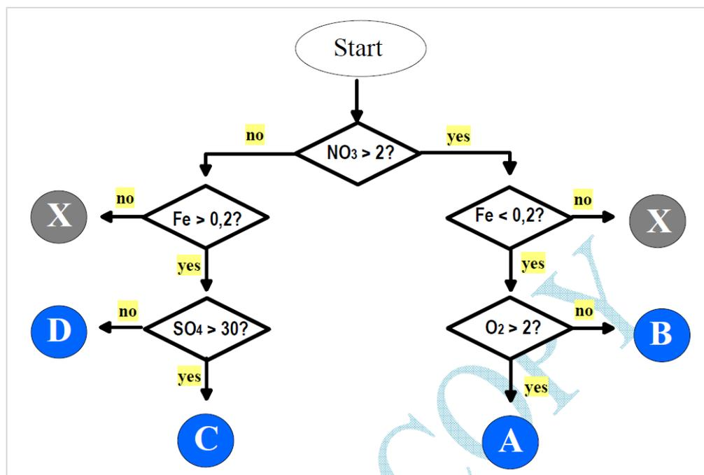
Figure 6.5 Algorithm for redox water type determination. (conc. in mg/L).
