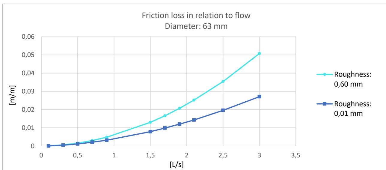
Figure 8.9 Friction loss in relation to flow at different roughness, diameter of 63 mm.
