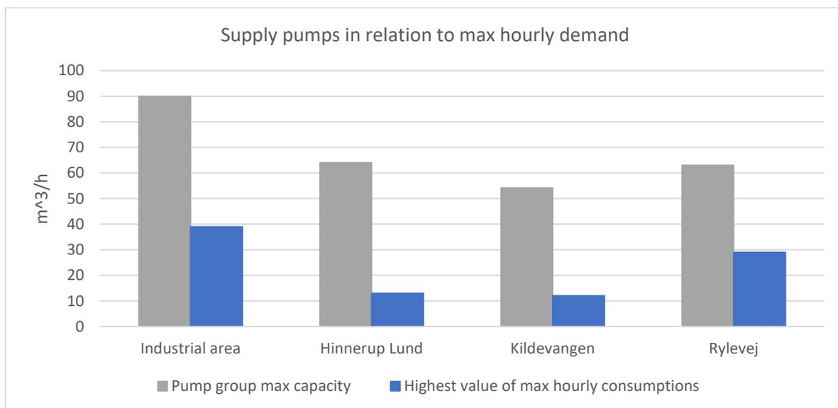
Figure 8.4. Maximum usage of the existent pumps with the assessed requirements.
