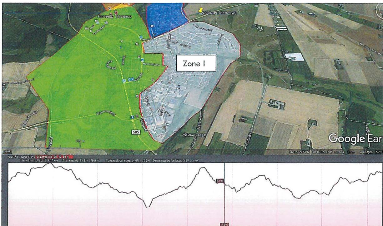
Industrial zone I, there is a level difference from level 59 to level 36, equal to an elevation difference of 23 meter.
