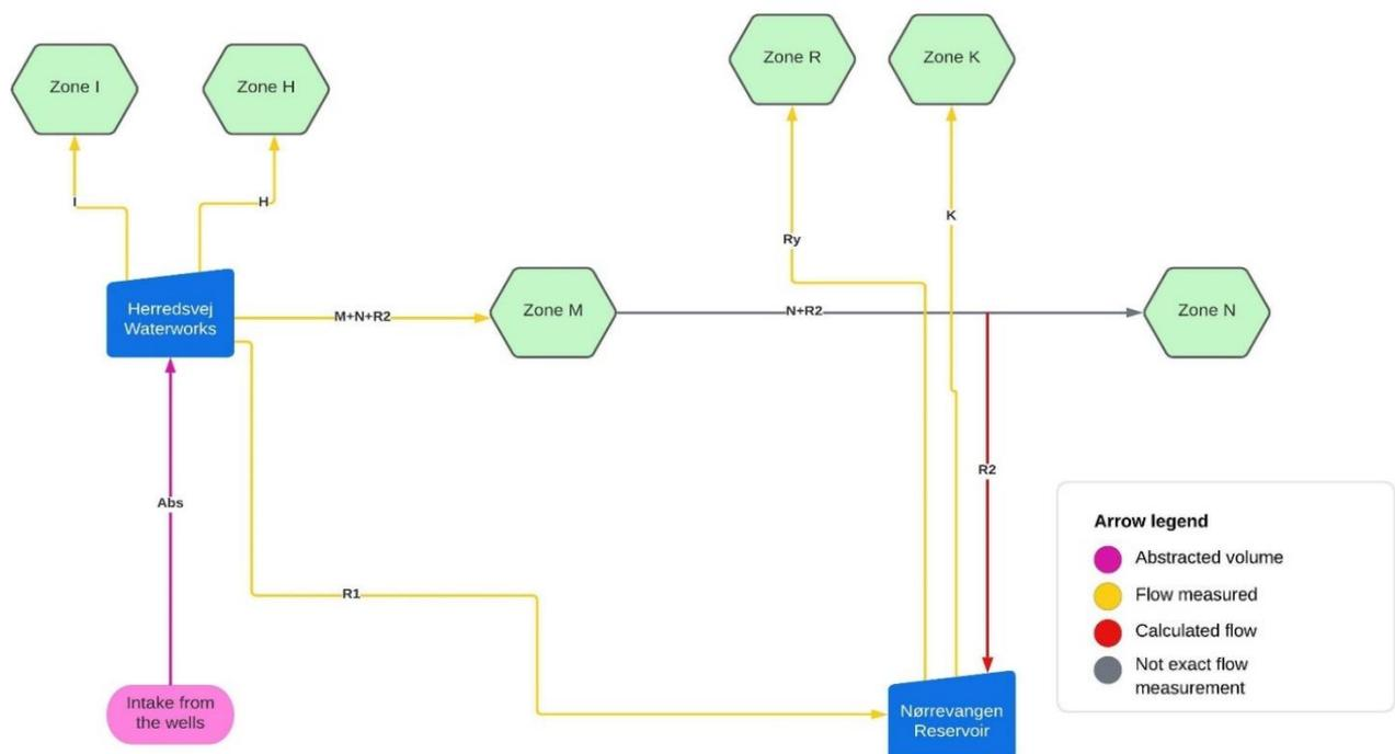
Figure 8.1. Overview diagram of the complete distribution network and denomination of the flows.
