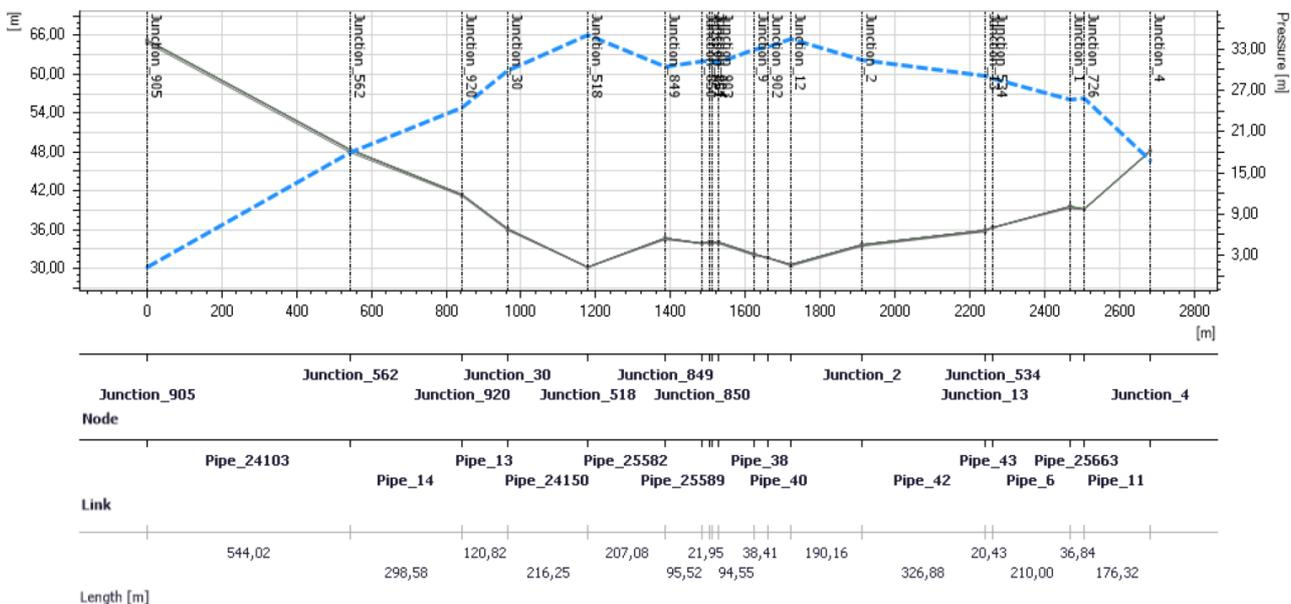
Figure 8.19 Profile plot of change in pressure. Water moving from main supply pipe to identified critical discharge point within the zone.
