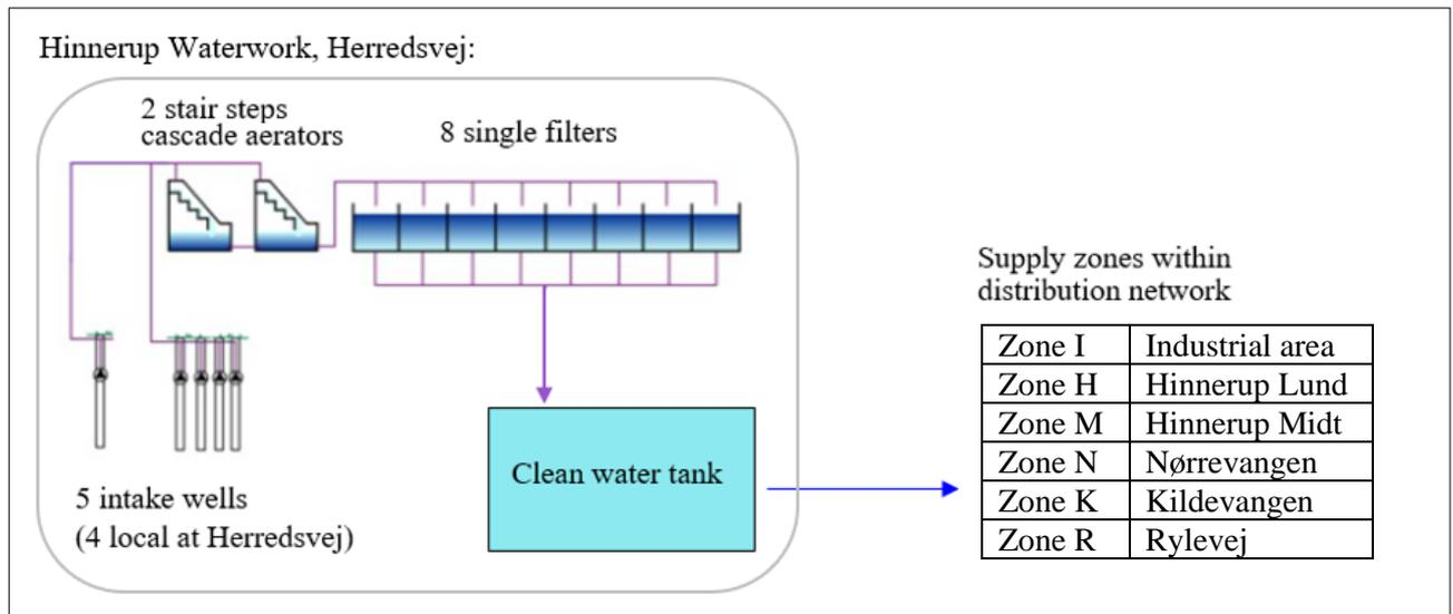
Figure 5.4 Simplified diagram overview of the complete supply system of Hinnerup.
