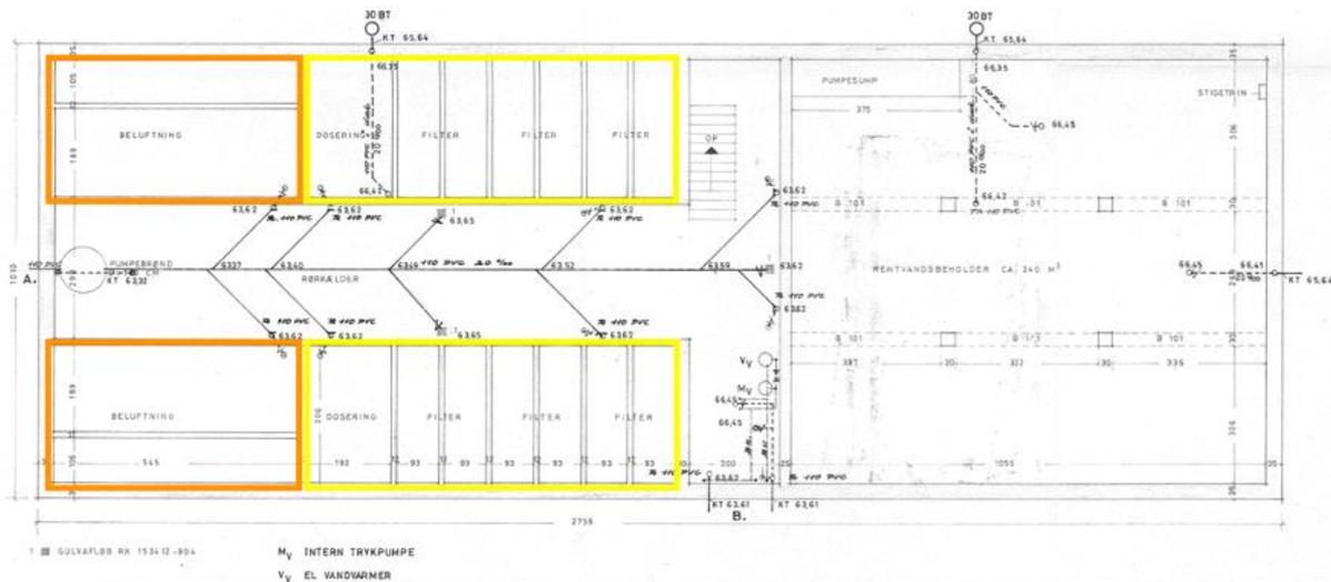
Figure 7.6 Schematic drawing of the floor plan in the Hinnerup waterworks. The orange marked areas are the Cascade aeration. In yellow the Sand filters can be seen. The drawing is from 1973. Since then, the "Dosing" has now also been converted into a sand filter. Provided by the waterworks.
