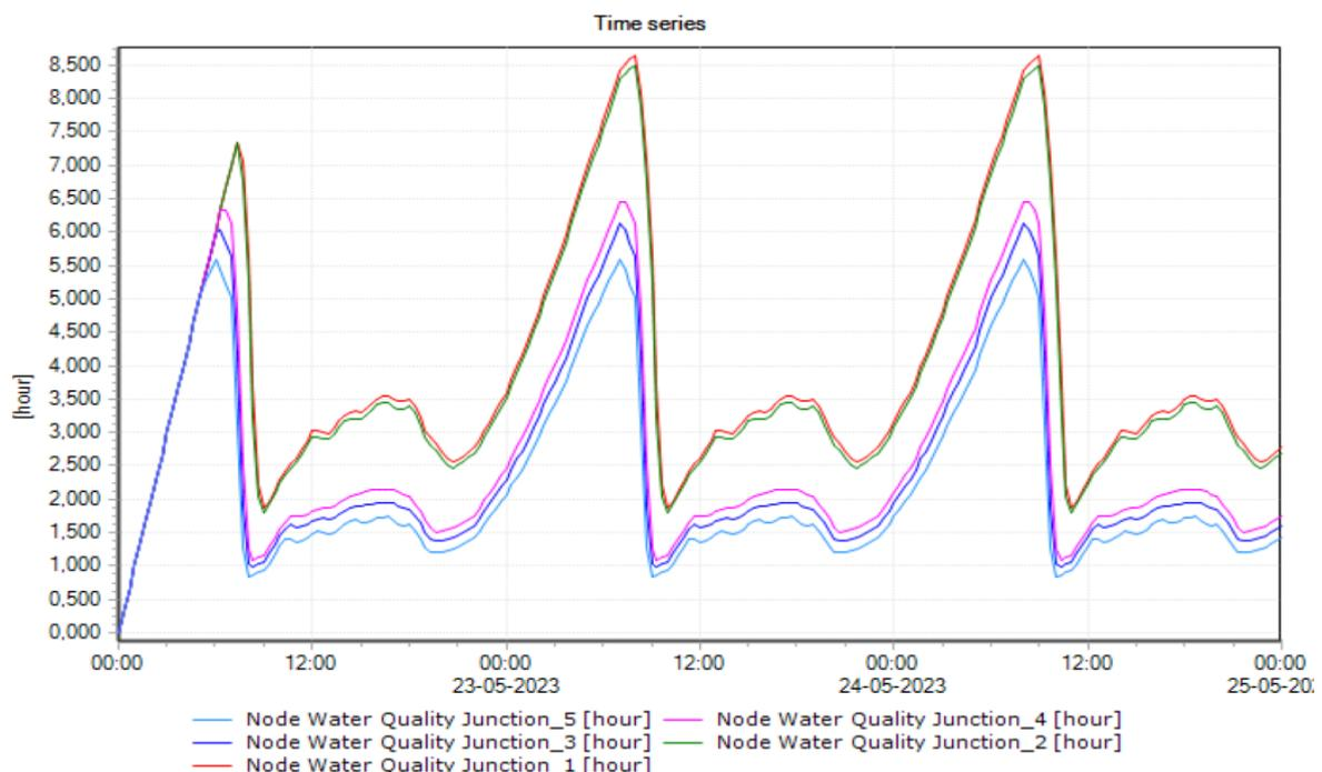
Figure 9.7 Graphical view of maximum residence time of critical discharge points within the future zone F
