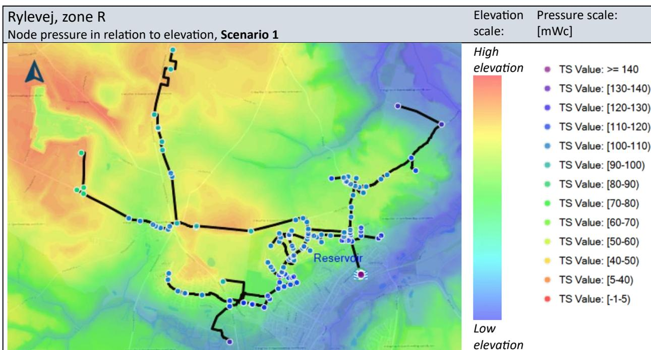
Figure 8.15 Rylevej, zone R, node pressure in relation to elevation, Scenario 1
