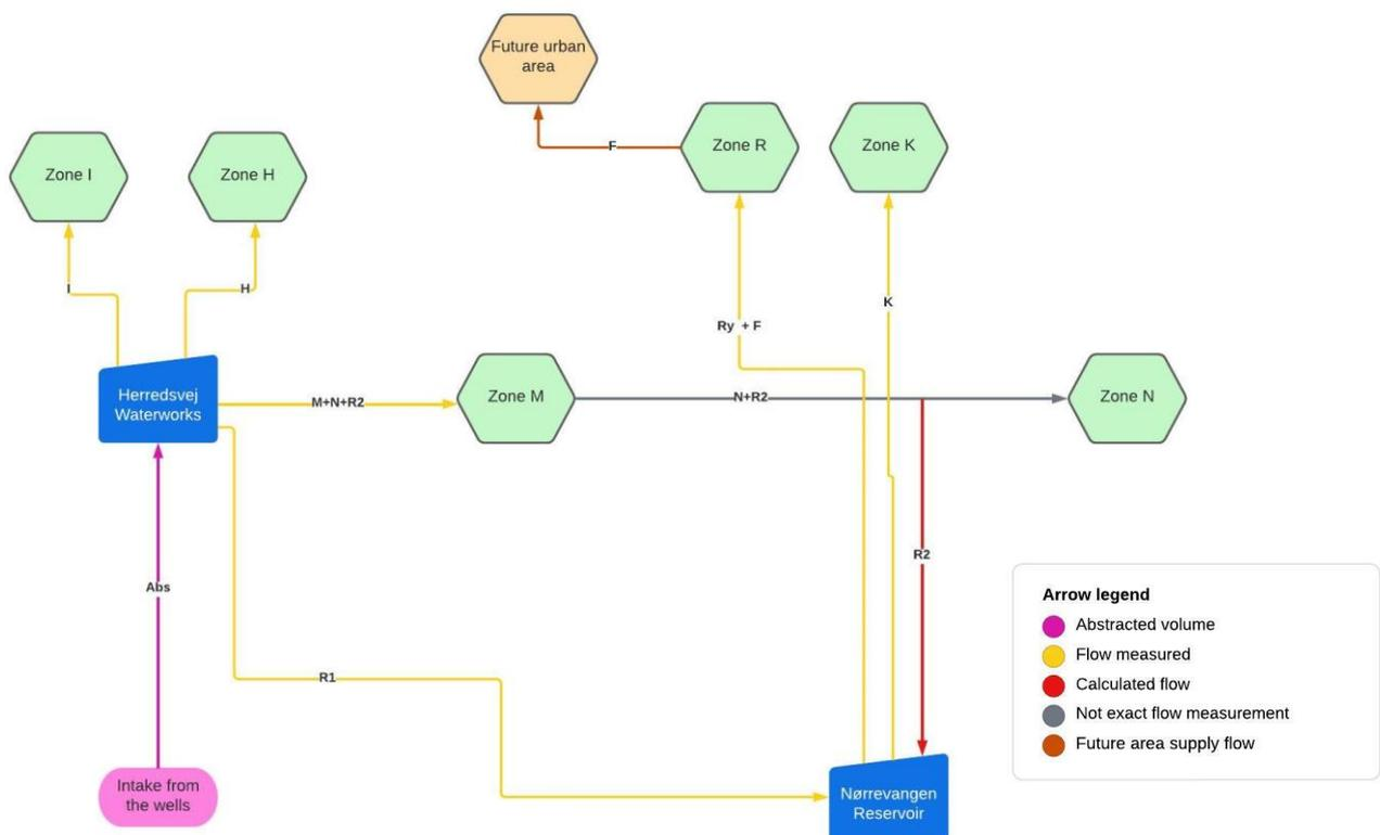
Figure 9.1. Flow diagram for the future distribution system.
