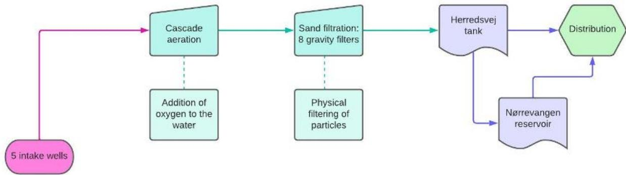
Figure 7.4. Overview diagram of the standard treatment and the way to the distribution system in Hinnerup.
