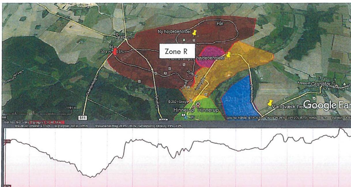
Rylevej zone R spån from level 78 to level 38, equal to a difference in altitude of 40 meters.
