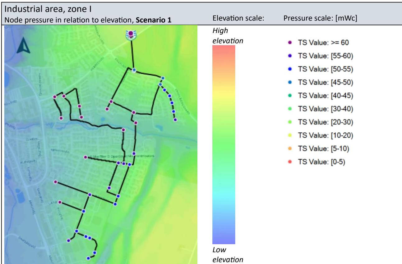
Figure 8.12 Industrial area, zone I, node pressure in relation to elevation, Scenario 1
