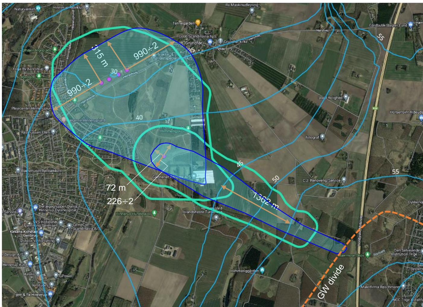
Figure 6.3 Drawing of the abstraction area based on calculations and in relation to the potentiometric surface map lines.
