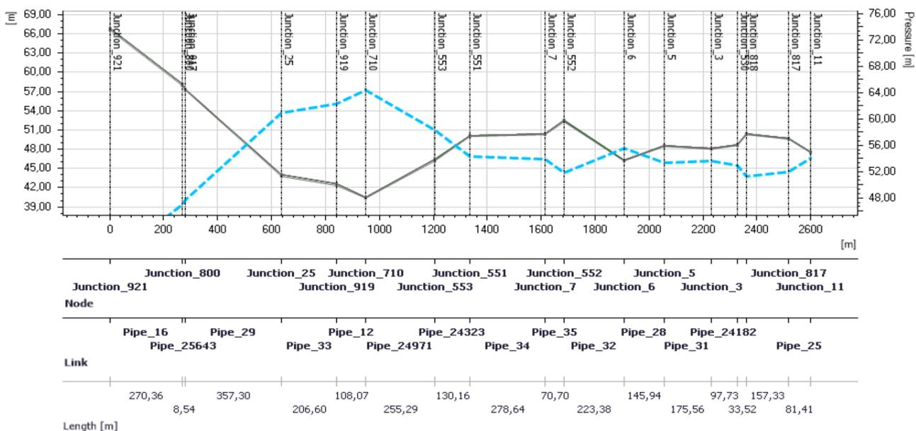
Figure 8.18 Profile plot of change in pressure. Water moving from main supply pipe to identified critical discharge point within the zone.
