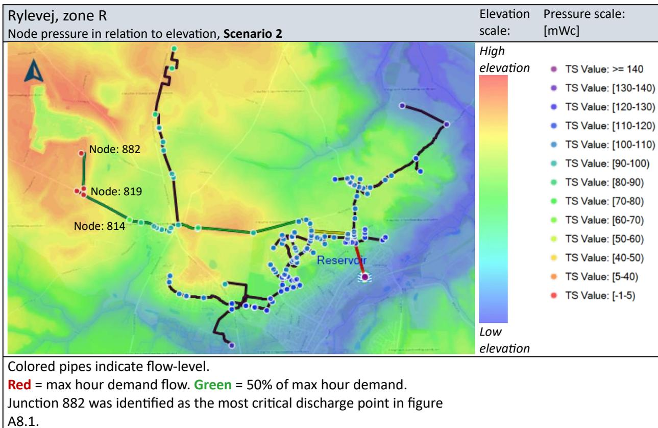
Figure 8.16 Rylevej, zone R, node pressure in relation to elevation, Scenario 2
