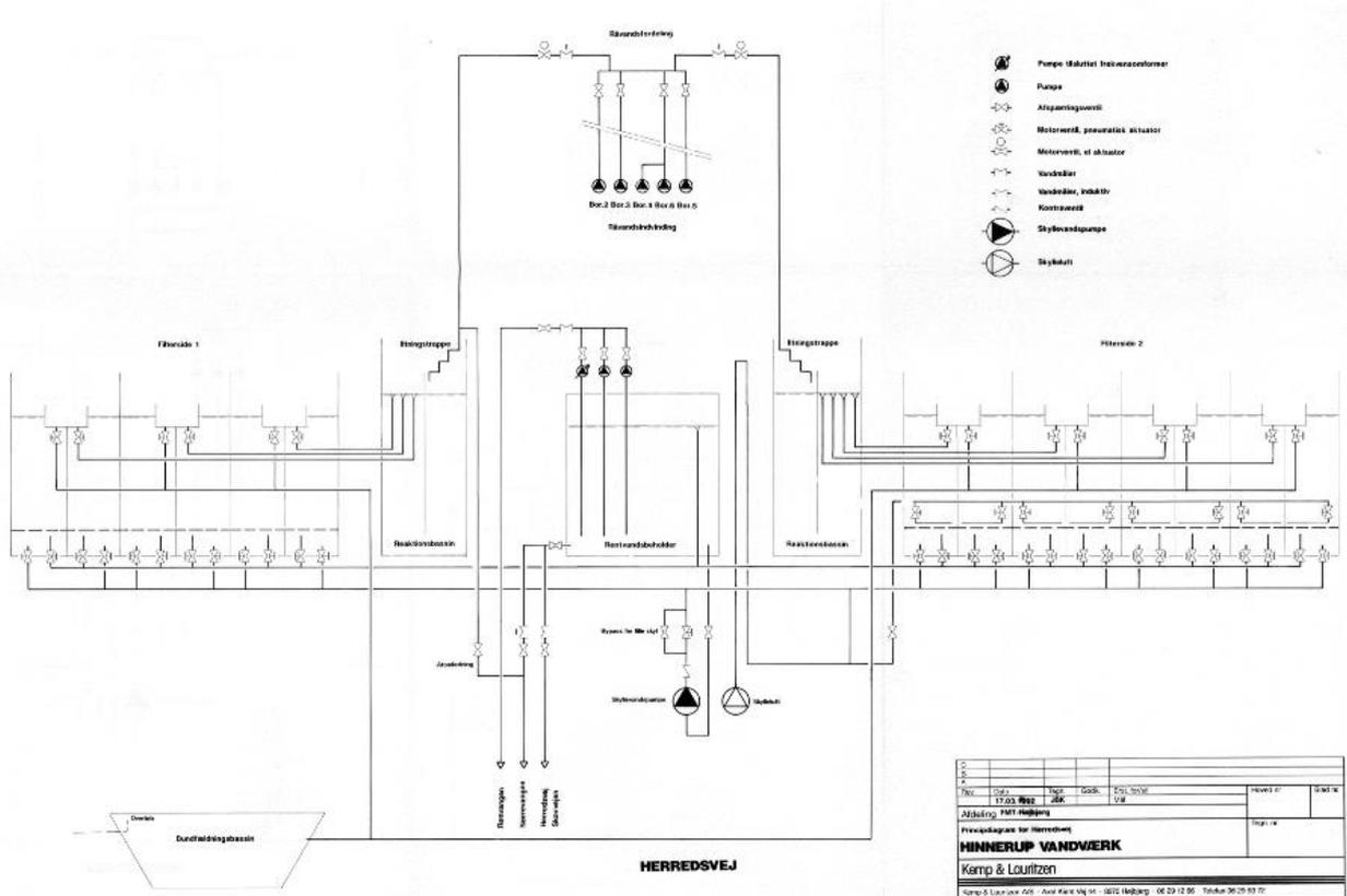
Figure 7.7. Pipe and process Diagram of the waterwork in Hinnerup from 1992 provided by the waterworks.
