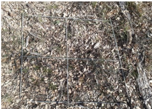
Figure S.M.2.5. Quadrant to measure leaf litter and herbaceous cover in forest plot 3.
