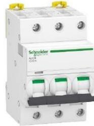
Magnetotérmico, Acti9 iC40N, 3P, 25 A, C curva, 6000 A (IEC 60898-1), 10 kA (IEC 60947-2)
