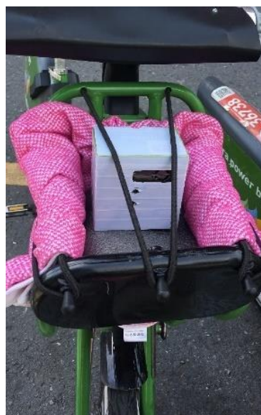
Figure 3. The developer's idea was to attach the device to a bicycle and gather data while cycling. However, since the tool is still a prototype, the tool was attached by improvisation to the bicycle basket, which made it difficult to keep the device safe while maintaining the air flow to the sensors.
