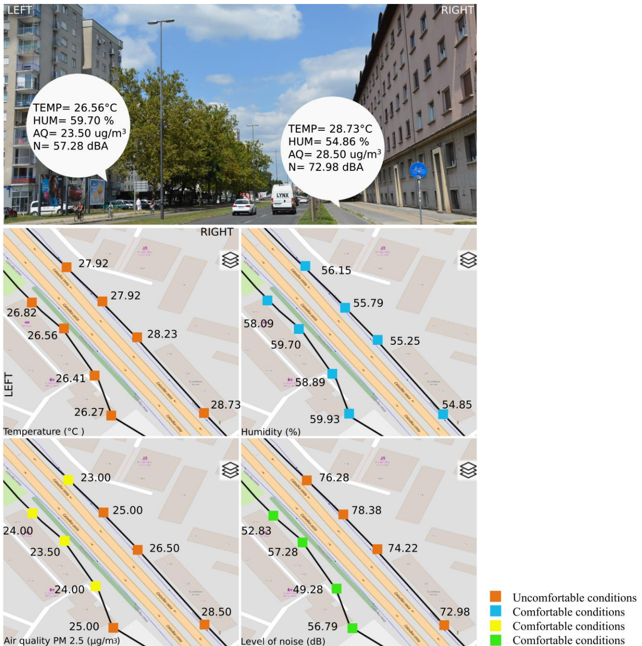
Figure 7. Microclimatic conditions of the left and right cycling lanes (Ljubljana, Friday, 23 July 2021, between 15:00 and 16:00). See the legend to interpret microclimate data in relation to human comfort values, represented with different colours (Table 1).
