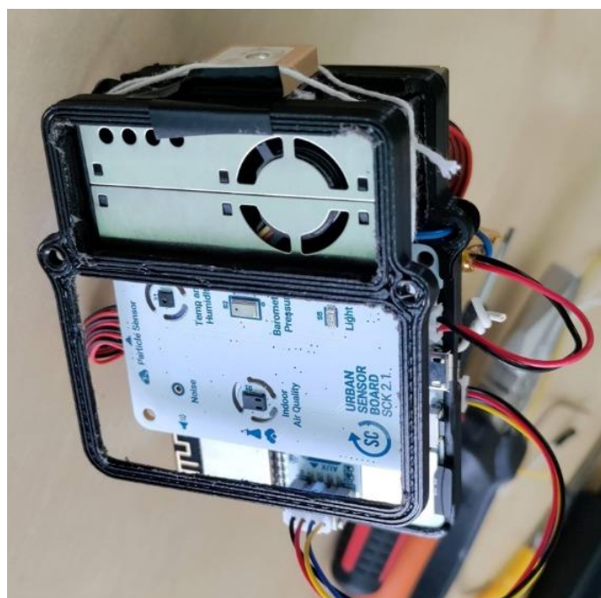
Figure 2. Hardware consists of environmental sensors and a GPS antenna.
