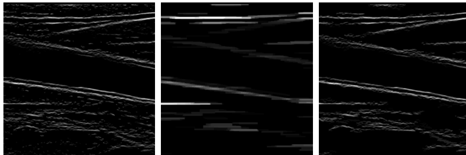
Figure 9: Mask (left), marker (centre) and reconstructed (right) images.
