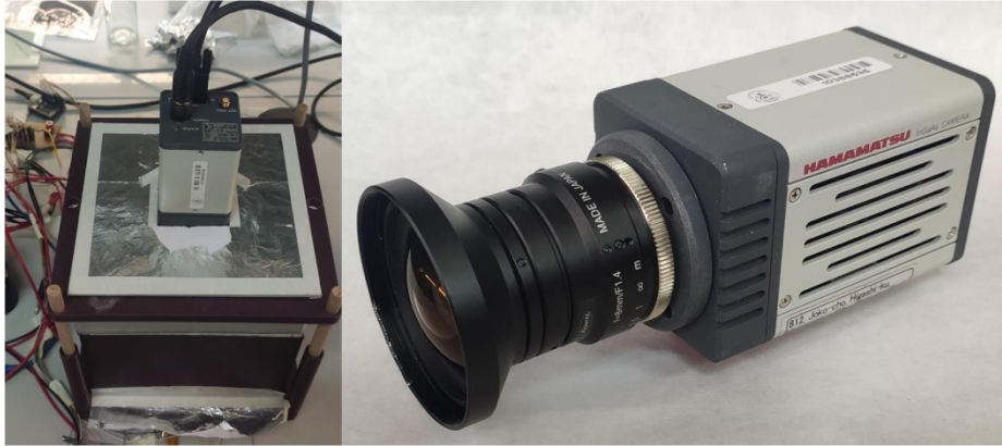
Figure 4. InGaAs camera, Hamamatsu brand and C12741-11 model, for EL imaging.
