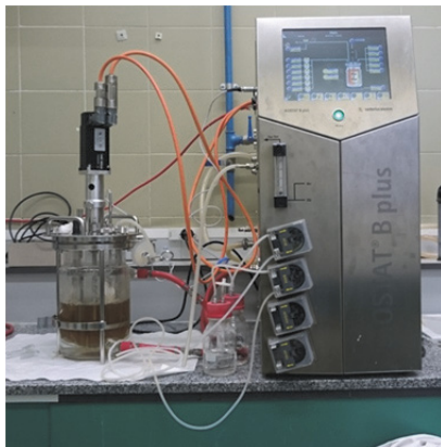
Figure 1. ABE fermenter with control equipment.
