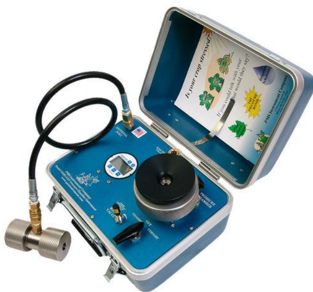
Figura 12. Cámara Scholander modelo M 1505D. https://mmm-tech.de/media/com_eshop/products/resized/m-1505d-exp-500x500.jpg
