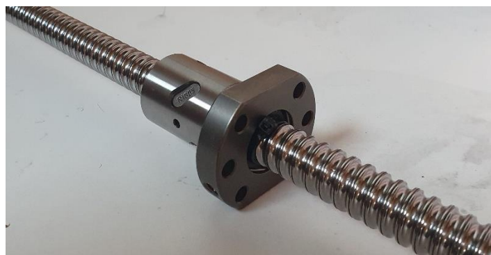
Figura 33 Husillo HBS1605RC7L1200 y tuerca DIN69051 [Imagen propia]
