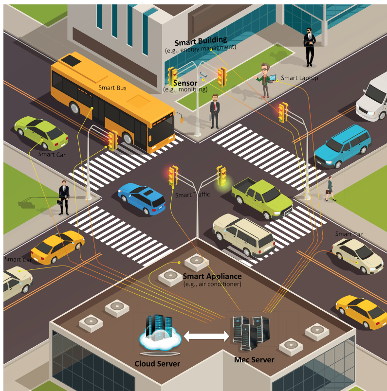
FIGURE 1. Network architecture of "Mobile Edge Computing".
