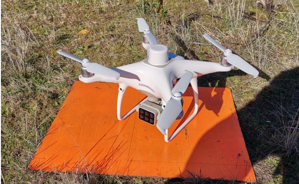
Figura 18: DJI Phantom 4 multispectral.
