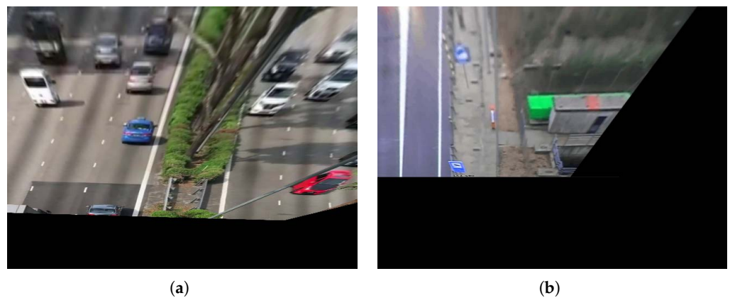
Figure 13. Examples of scenarios with corrected perspective. (a) Scenario No. 6. The perspective has been corrected for the most part. (b) Scenario No. 7. The perspective has been satisfactorily corrected.
