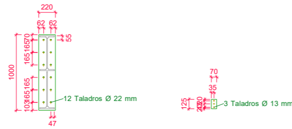
Chapa frontal de la viga (a) IPE 450 (e = 15 mm) Chapas laterales (e = 8 mm)
