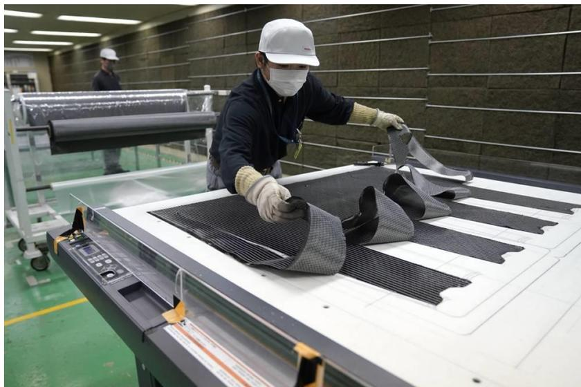
Ilustración 68. Guangzhou Wise (2020) Operario cortando láminas de fibra de carbono. [fotografía] China <https://www.gdwise.com/info-detail/ns-showcases-new-cfrp-process-that-reduces-moulding-times-by-up-to-80-5>
