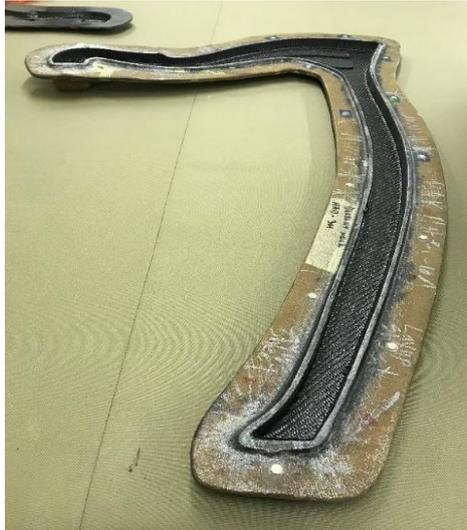
Ilustración 65. Molde de fibra de carbono para arpa Legend. 2012. Heartland harps. <https://heartlandharps.com/harps/models/>
