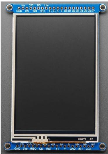
Figura 134 Adafruit 3.5" TFT LCD touchscreen – HXD8357D. Vista frontal.
