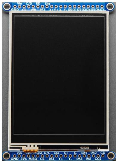
Figura 131 Adafruit 3.2" TFT LCD touchscreen – ILI9341. Vista frontal.
