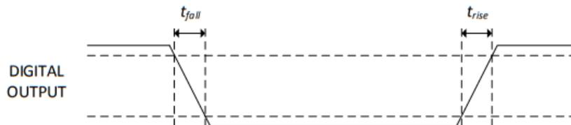
Figure 2: Digital IO Characteristics
