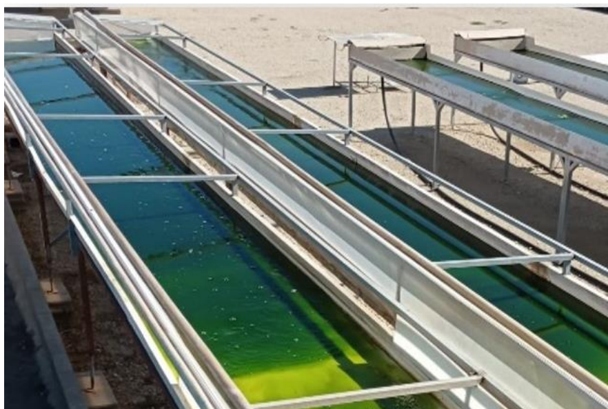
Figure 9.1. Scheme of the microalgae-bacteria treatment of the diluted liquid fraction of swine manure (up) in a pilot scale thin layer photobioreactor in IFAPA facilities at University of Almería (down)
