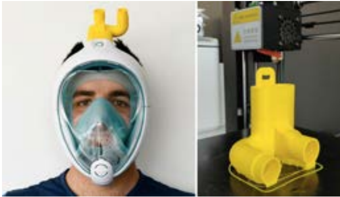
Diving mask transformed into a respirator (photo credits: Isinnova)
