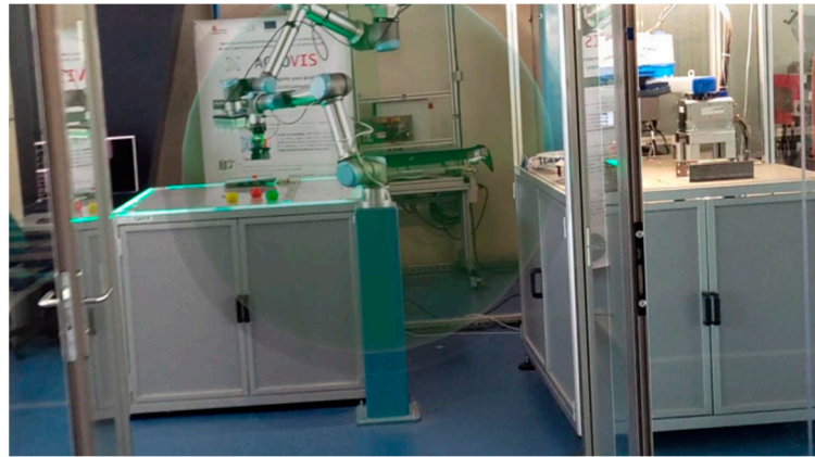
Figure 7. Visualization of the cobot workspace. Screenshots of the application during its execution.
