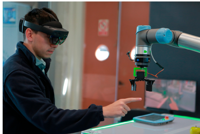
Figure 4. User interacting with the UR5e through Microsoft HoloLens 2.
