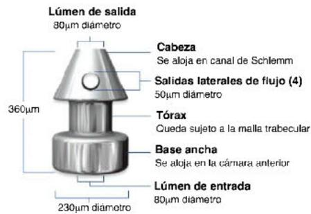
Figura 1. Dimensiones del iStent inject. Berdahl, J. (2019, September/October). *Istent inject versus iStent: The iStent inject advantage. Glaucoma Today.* <http://glaucomatoday.com/2019/10/supplement2/istent-eminjectem-versus-istent-the-istent-eminjectem-advantage/>
