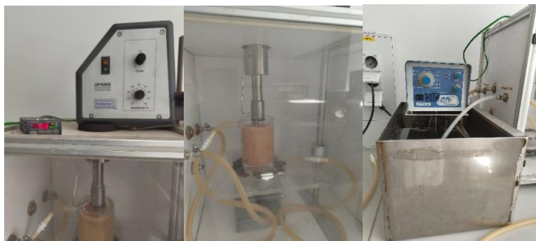
Figure 2. UP400S processor (Hielscher Ultrasonics GmbH, Teltow, Germany) with the sample and the water bath (Selecta Tectron 200).
