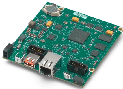
Figura 3.3: Controlador sbRIO 9607 de National Instruments.
