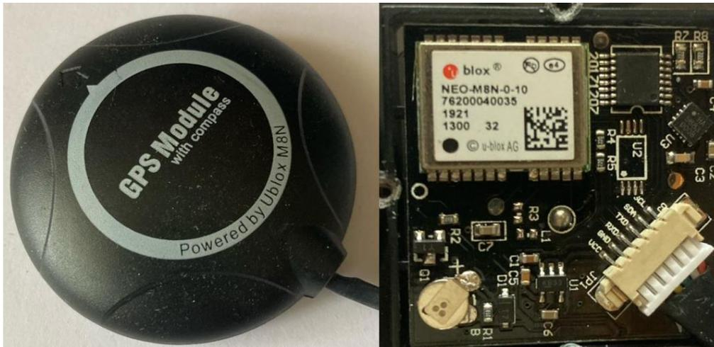
**Figura 39.** Sensor GNSS NEO-M8N.
