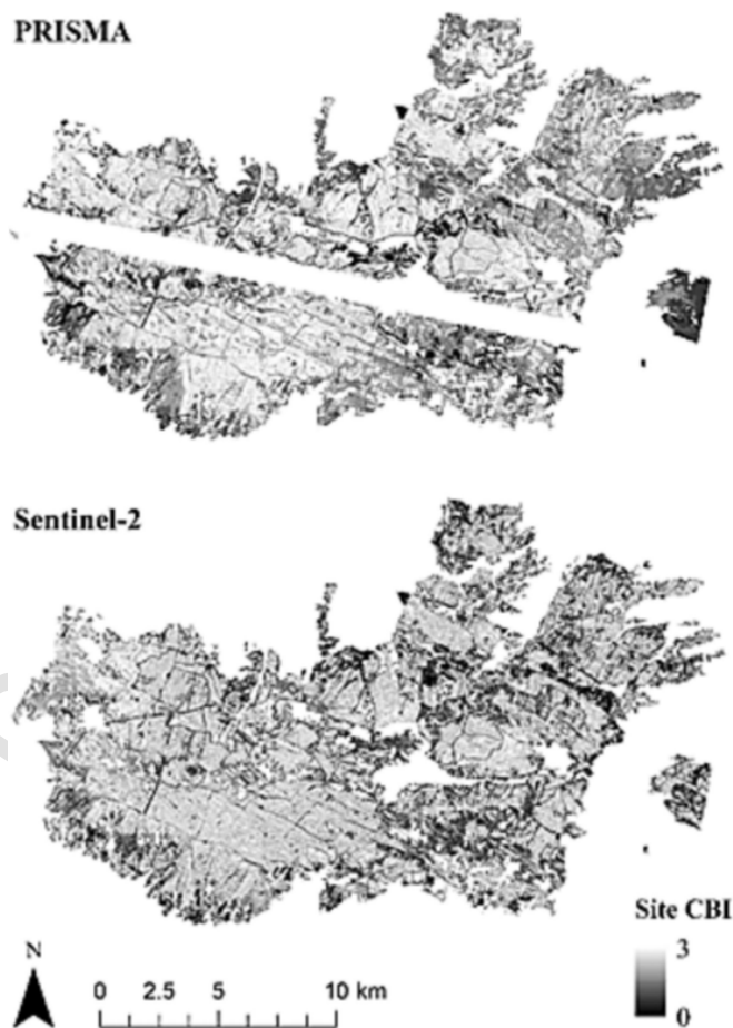
Fig. 5. Composite Burn Index (CBI) maps computed from Random Forest regression (RFR) model outputs for Sentinel-2 and PRISMA.
