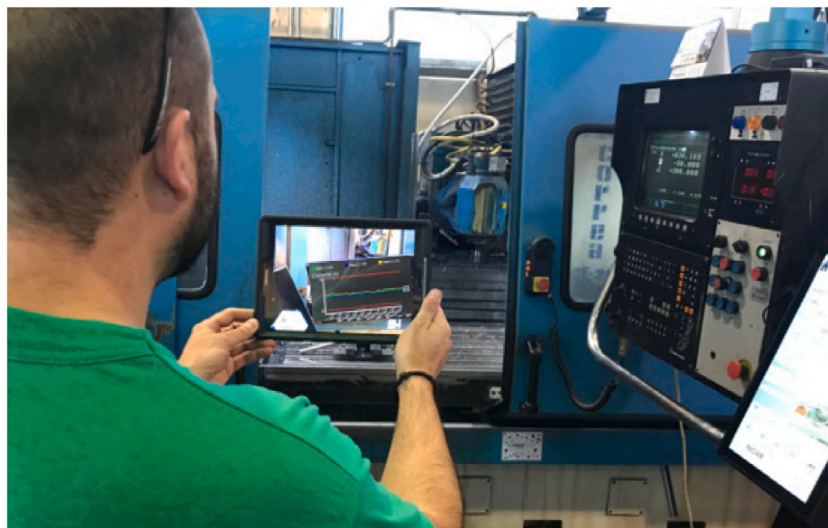
Fig. 8. Worker putting into practice augmented maintenance operations by detecting abnormal start-ups of a legacy milling machine.
